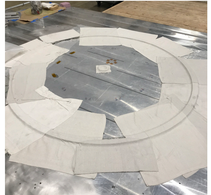
Vacuum lamination of G10 and lead.
