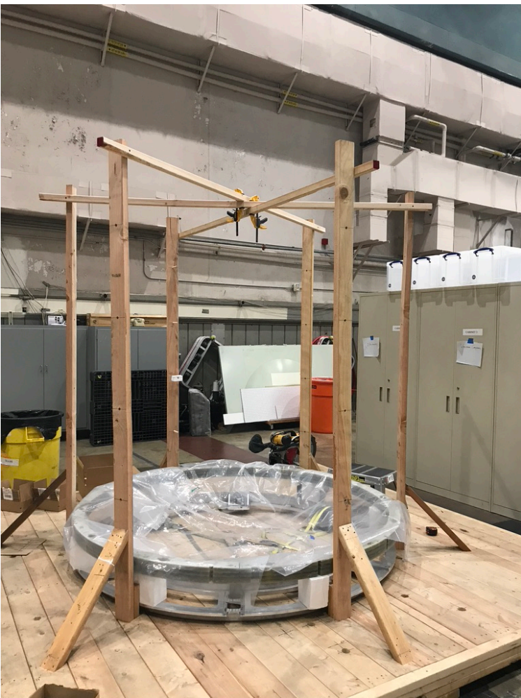
Wood structure to support the B0 magnet core assembly.
