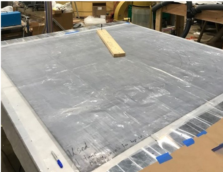
The annular lead rings are cut from a 90"x90" sheet of lead using scissors, chisels and piano wire.
