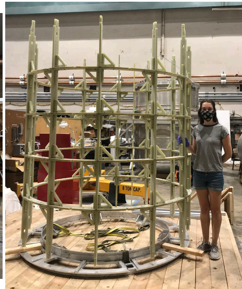
B0 magnet core assembled with Alina Aleksandrova for scale!
